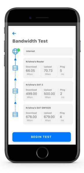
To run a bandwidth test simply select the "Begin Bandwidth Test" button at the bottom of the screen. The speed test will first run between the GigaSpire and the Internet and then will conduct a speed test between any mesh units and the GigaSpire. Results will show as a notification, update at this location, and on your main dashboard.
