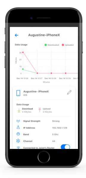
The device details screen will show the device name at the top of the screen followed by a chart that indicates the amount of date that was used by the device over a period of time.
